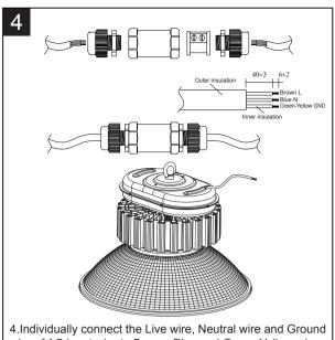
4.Individually connect the Live wire, Neutral wire and Ground wire of AC input wire to Brown, Blue and Green-Yellow wire. All cable teminations must be installed in accordance with the designed IP rating.
